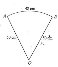
The diagram shows a sector of a circle with centre O and radius 50 cm. The length of the arc AB is 48 cm.
